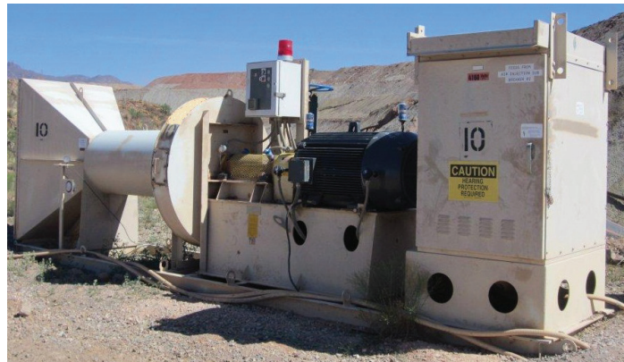
Mine shaft pressurization (above); single skid mounted inlet filter box, silencer, blower assembly, disconnect and power supply drive. Multiple units, shown below, during factory assembly.
